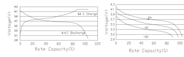
7.2 Charge/Discharge Cycle Life Charge:CC/CV 4.2V% 0.5C₅mA, E nd-Current 0.01C₅mA Discharge:0.5C₅mA,Cut-off at 3.00V T emperature:25!
