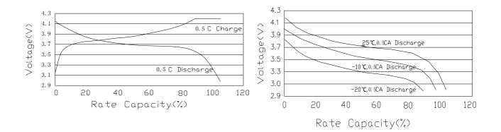
7.2 Charge/Discharge Cycle Life Charge:CC/CV 4.2V, 0.5CA, End-Current 7mA Discharge:0.5CA,Cut-off at 3.00V Temperature:25°C
