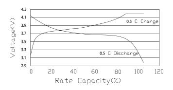
7.3 Temperature Characteristics Charge: CC/CV 4.2V 0.5CA,End-Current15mA
